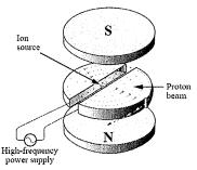
Ernest Lawrence was the first person to use a cyclotron. His cyclotron accelerated protons to a maximum energy of  $8.0\times10^4\,\mathrm{eV}$ . With this energy, the protons moved in a circular path with a radius of  $6.5\times10^{-2}\,\mathrm{m}$ .
